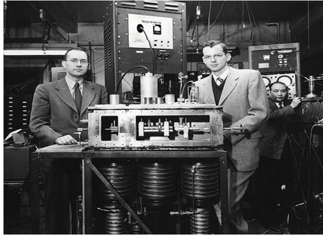
Şekil 2.2: İlk lazer cihazı - M.A.S.E.R (Microwave Amplification by Stimulated Emission of Radiation) - Charles Townes ve M.A.S.E.R., 1947
